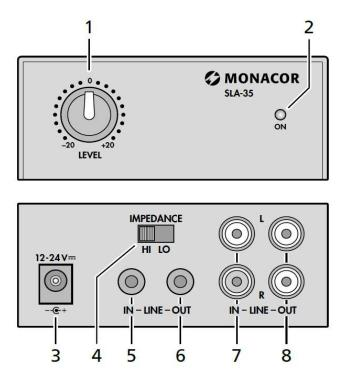
Connect the line-output of the A series, RM series or other PA amplifier to the twin phono inputs (7) of the SLA-35
